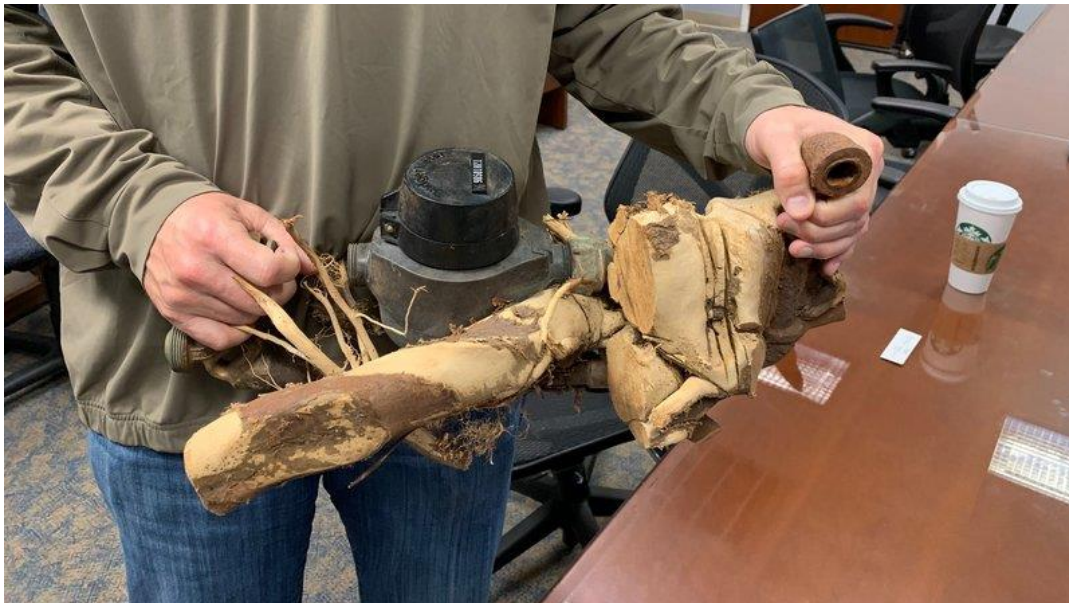
Paradise Irrigation District manager Kevin Phillips shows a sample of the town's water pipes, which were frequently woven between underground root systems that were likely burned during the fire. Kirk Siegler/NPR
